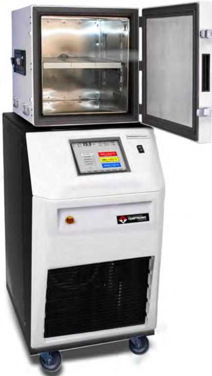
MOBILETEMP™ system configured with Front Load style THERMOCHAMBER™ connected via "Direct Dock" to a THERMOSTREAM® temperature source
